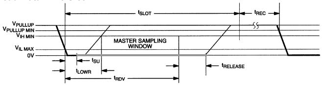
$\mu$ s  $\leq$   $t_{SLOT}$  < 120  $\mu$ s  $\mu$ s  $\leq$   $t_{LOWR}$  < 15  $\mu$ s  $\leq$   $t_{RELEASE}$  < 45  $\mu$ s  $\mu$ s  $\leq$   $t_{REC}$  <  $\infty$   $t_{RDV}$  = 15  $\mu$ s  $t_{SU}$  < 1  $\mu$ s
